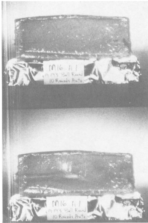
FIG. 6a—M16 in full automatic mode: Two consecutive frames from the Hycam 16-mm high-speed motion picture show: early penetration (top) and 4-in. (10.2-cm) long tubular "neck" region and tilted ellipsoid configuration of the emerging temporary cavity in the zone of bullet breakup (bottom).
